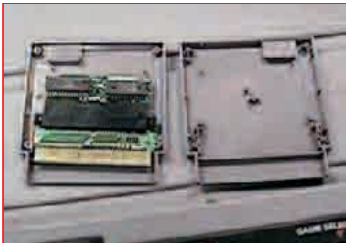
The famed Famicom-adaptor-in-a-NES-cart, which can be found in a few American NES games
