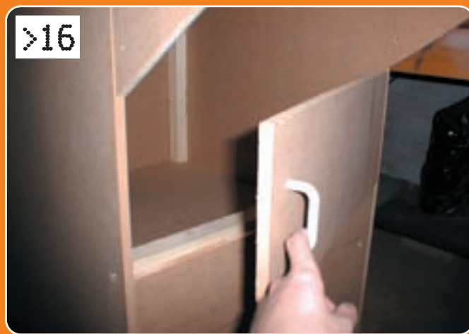
>16 The front door is next. This is a panel attached with a couple of hinges, with two wooden batons running across inside the case so that it doesn't spring back too far and end up inside the case. The handle is a standard draw handle, bought cheaply from a DIY store.
