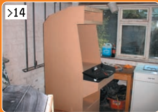
>14 Next, more cross-pieces are added at the top (directly above and below where the arcade cabinet's marquee will eventually live). At this point, the plan is to have the marquee attach to these wooden batons, so they're mounted flush with the front of the cabinet.
