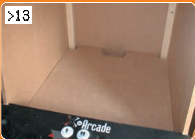
>13 Two internal shelves are next - one for the PC components and one for the monitor. These are supported underneath by batons screwed into the front and back of the cabinet. We've taken a chunk out of each shelf at the rear, to enable cables to be threaded through.
